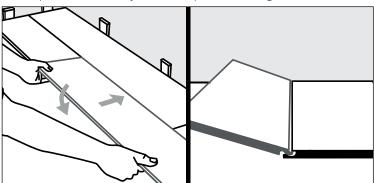
and lightly tap on the top of the flooring being installed near the joint seam. You
