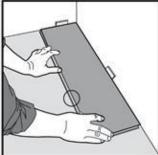
4. Install the second row by aligning and dropping the end tongue over the end groove of the first piece. Apply light pressure to join the two pieces together.
