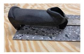
Do a test cut on the tile to check the depth of your groover tool on a sample piece of tile.
