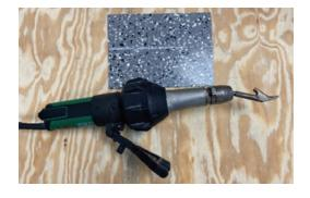
Practice on a test piece to get the temperature and speed correct.
