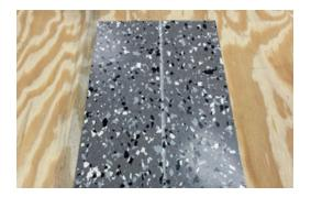
Create a seam weld sample to experiment on achieving the optimum melt flow for your floor conditions.
