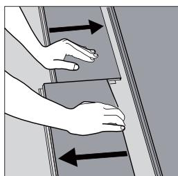
Separate the whole row by lifting it up delicately at an angle. To separate individual plank end-joints within a row, leave them flat on the ground and slide them apart. If planks do not separate easily, you can slightly lift up the planks (5°angle) when sliding them apart.
