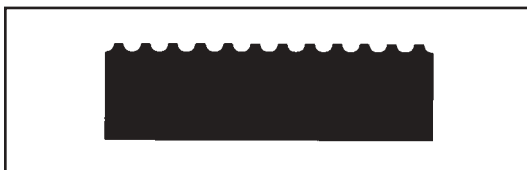
Fig. 7 - Required trowel notch size.
